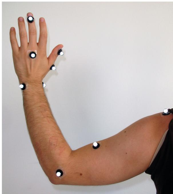
Fig. 1: VICON marker set. One marker (on ulna styloid process) is hidden.
